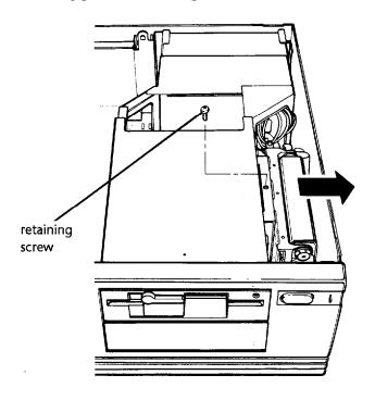
3. Tilt the hard disk drive slightly to the right, away from the subassembly, and lift it out of the vertical mounting area. Turn it over and set it on top of the subassembly with the gray mounting plate facing up. Since the drive is attached to its cables, make sure you do not try to move it too far away from the subassembly as you turn it.
